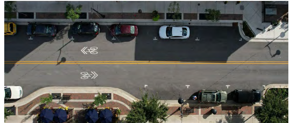
Example of On-street Parking Space Delineation
