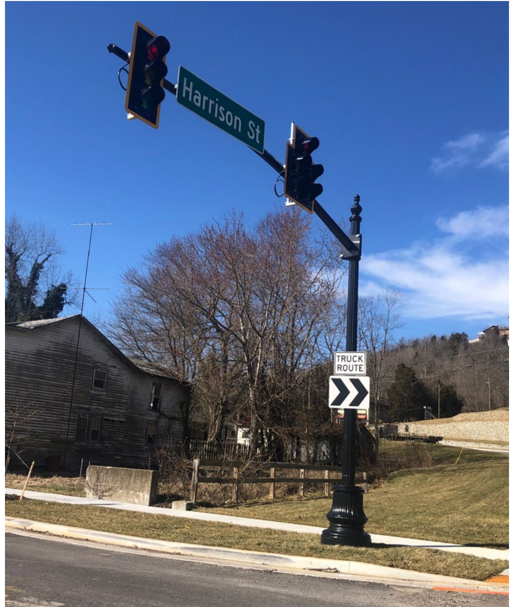
Project 421 black decorative metal mast arm traffic signal. Design intent for Main Street is to match.
